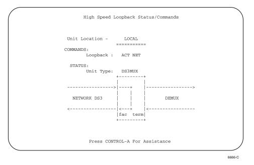
Note: Do not perform a DS3 loopback when the Soneplex Broadband chassis is connected to a DS3 CAM unit in the Soneplex CCAS system.
